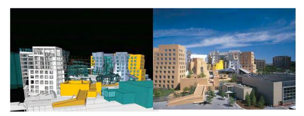
The final CATIA 3D construction model offered detailed representations of five structural elements: concrete, structural steel, exterior skin, framing, and assembly patterns. While concrete was being poured and placed on site in Cambridge directly from the 3D model, the structural steel was being fabricated, by Capco, Corp. in Rhode Island using a 2D translation from the model. The metal and glass for the skin were also being fabricated off-site directly from the 3D model using CNC technology.
